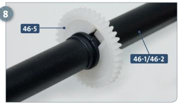
Slide the gear **46-5** down the shaft cover **46-1/46-2** until it sits against the bead. Pay close attention to the gear's alignment.
