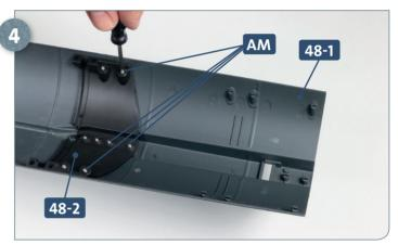
Fix the lower hull section **48-1** to the main hull structure using four **AM** screws in the holes in the connector **48-2**.
