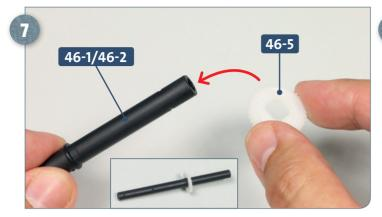
Now fit the cog **46-5** onto the end of the shaft cover assembly **46-1/46-2**, as shown in the inset photo and in the next step. Note the distance from the end of the shaft to the rib is shorter.
