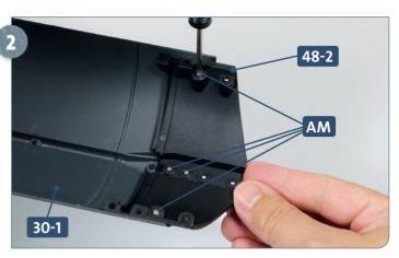
Fix the connector **48-2** to the lower hull section **30-1** using the four **AM** screws.
